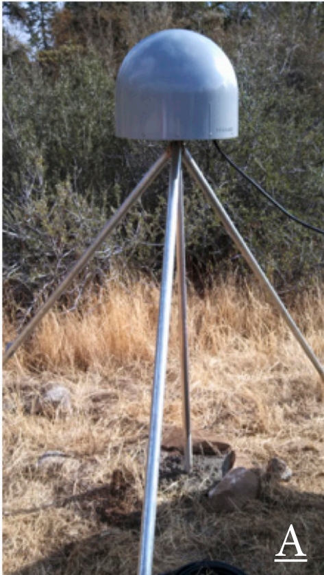
Figure 4.6.3: A) Photo of station HELB showing completed monumentation. B) Phase residual plot from daily processing for HELB on 1/8/2014. This shows the goodness of fit for observations throughout the day. Small excursions from the red lines (orbit tracks) indicate phase measurements that are well fit by a stable position. The plot is oriented such that the north direction is at the top.
