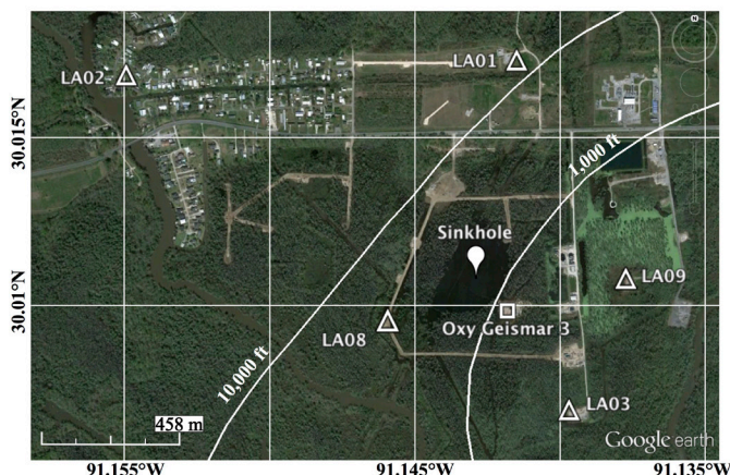
Figure 2.25.1: Google Earth Image (dated March 12, 2013) shows the study region at the western edge of NSD, with 1000 ft and 10,000 ft contours indicated by white lines, locations of the five USGS broadband stations (white triangles), approximate location of the Oxy Geismar 3 cavern (white square), and an average point location of the sinkhole (white balloon).
